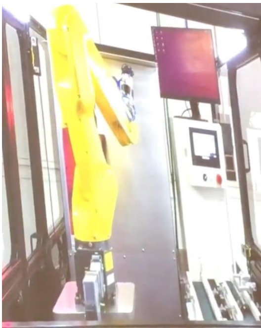
Figure 5. Automated Bevel Inspection using Cameras and GPUs
